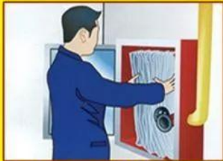
1、打开或击碎箱门，取出消防水带 Open or break fire-fighting hydrant door, take out water pipe
