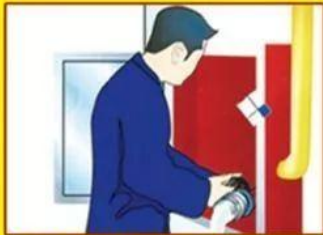
5、另外一人打开消防栓上的水阀开关 The other person opens the valve of fire-fighting hydrant
