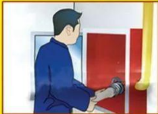
3、水带一头接到消防栓接口上 Connect one side of water pipe to fire-fighting hydrant
