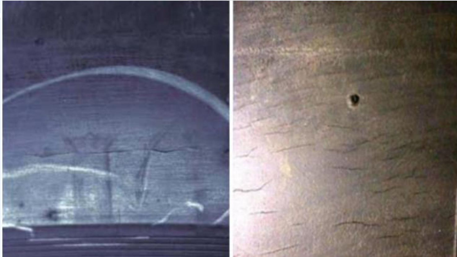
侧壁橡胶老化和裂纹
